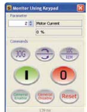
Monitoring and control window using virtual HMI
